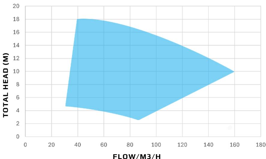
\*Pump performance curve is based on water with a SG=1.0 and without additional accessories.
